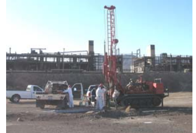
Soil sampling with hollow stem augers (Parcel F)
